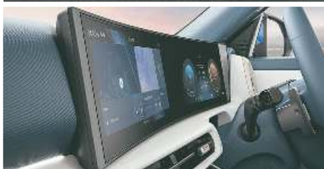
Dual 62.5 cm (24.2") x 12.3" curved panoramic display with Connected Car Navigation Cockpit (ccNC2) and Controller - OTA
